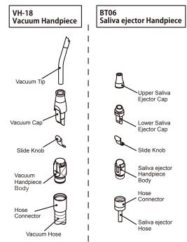
**Fig.5-7** Vacuum Handpiece and Saliva Ejector Handpiece
