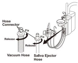
Fig.5-6 Vacuum and Saliva Ejector Hose
