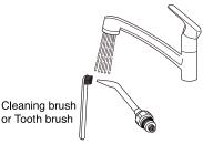
Fig.5-14 Cleaning Belmont 77 Syringe Nozzle
