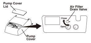
Fig.5-16 Air Filter Drain Valve
