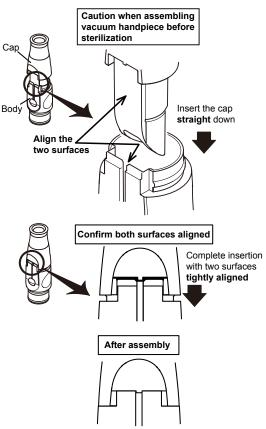
Fig.5-11 Assembly before sterilization (Vacuum Handpiece)
