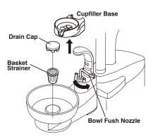
Fig.5-1 Drain Cap, Basket Strainer, and Cupfiller Base
