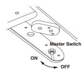
Fig.3-1 Master Switch and Indicator
