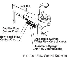
Fig.3-20 Flow Control Knobs in Cuspidor Unit Body C. Bowl Flush Flow Control Knob (Fig.3-20)
