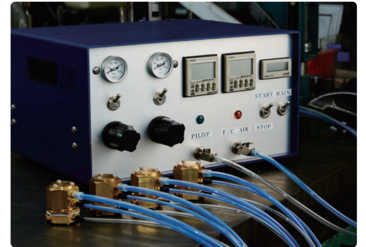
All valves undergo 1 million repetitions of durability testing.
