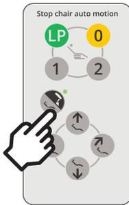
Membrane switches on the control panel (Rod)
