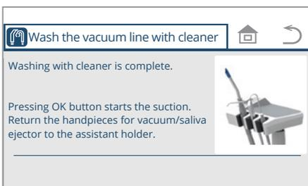
\* After the suction starts, return the vacuum and saliva ejector handpieces to the assistant holder. When the vacuum and saliva ejector handpieces are returned to the assistant holder, the screen returns to the home screen.
