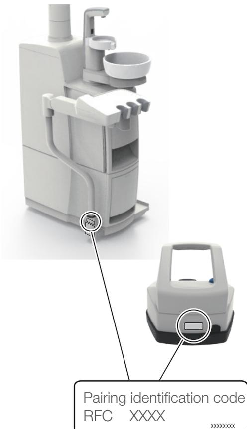
Operate the wireless foot controller within one meter of the product.
